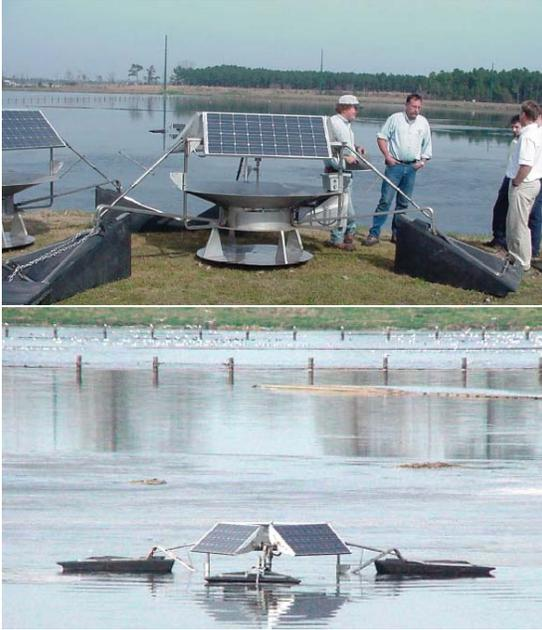
*Figure 7. SolarBee® installed in City of Myrtle Beach, South Carolina, 50-acre wastewater lagoon.*
