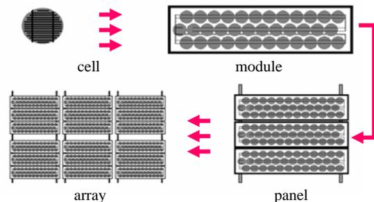
Figure 4. Solar module composed of individual solar cells.
