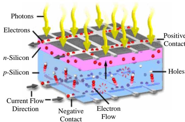
Figure 3. Electron and current flow in solar cell.
