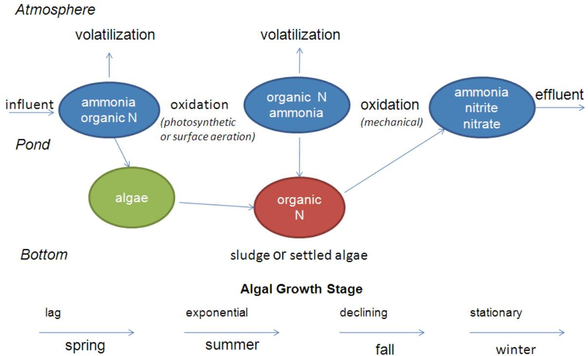
**Figure 1-1. The nitrogen cycle in wastewater pond system.**
